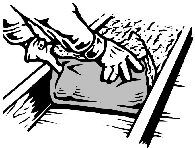
Figure 3. Correct installation of batt insulation
